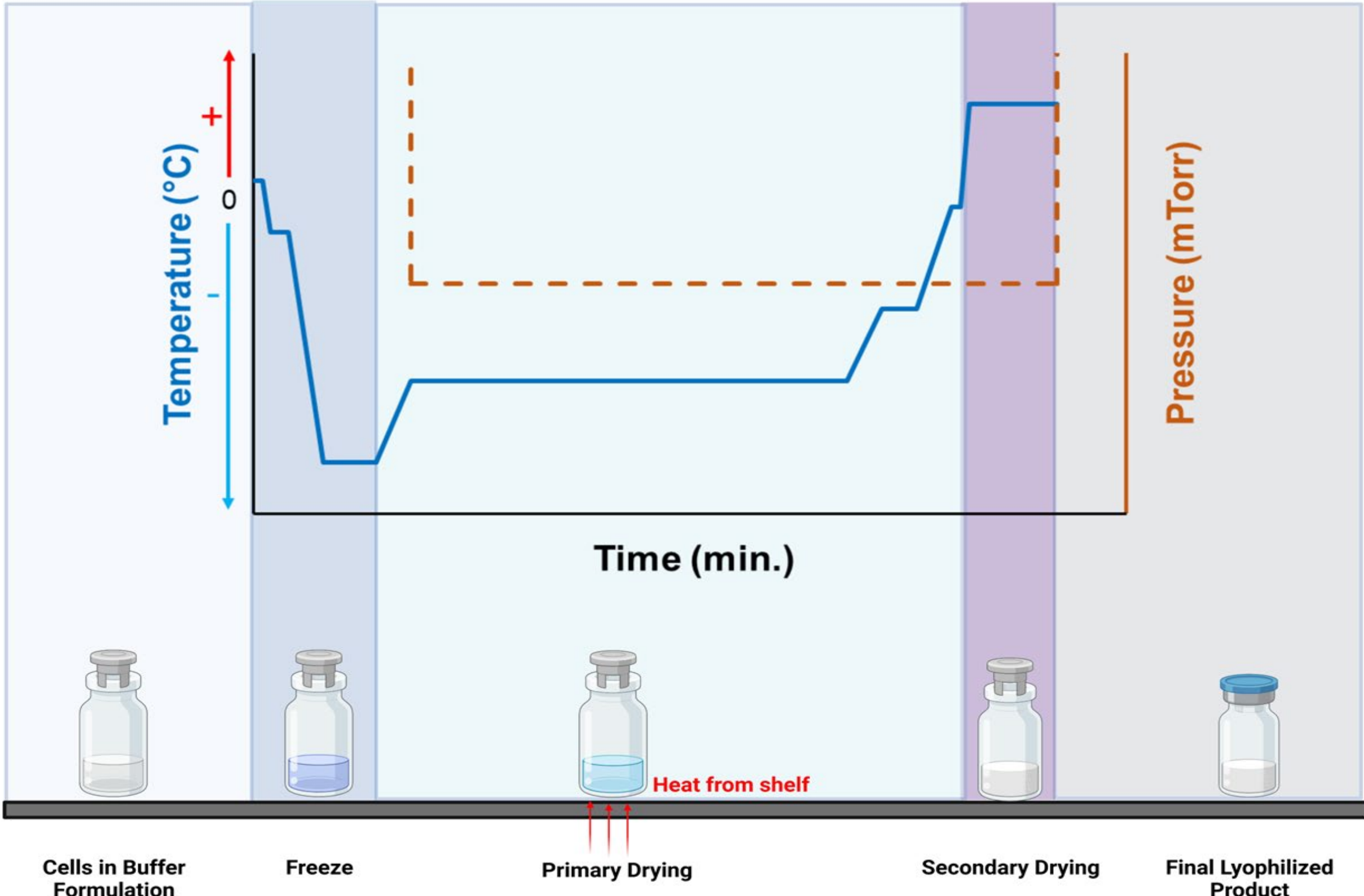
Figure 1: Overview of microbial lyophilization. The process allows ice to change from a solid to a vapor without going through a liquid phase. This process comprises three major steps: freezing the sample, primary drying (ice sublimation), and secondary drying (unfrozen water desorption).
